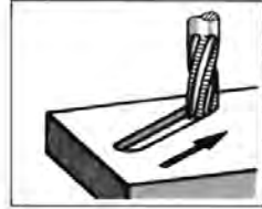
G01 LINEAR INTERPOLATION (STRAIGHT LINE MOVEMENT)
